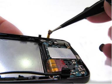
Using the fine pointed tweezers, unplug the cords connecting the headphone jack to the chip.
