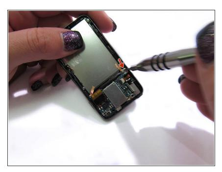
Unscrew the 1 screws around the headphone jack using Phillips PH000 screwdriver.
