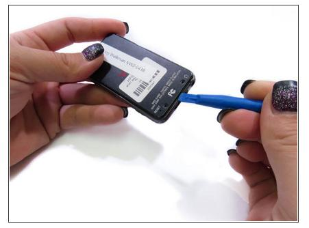
• Use a small prying tool to carefully pry open the back of the device.
