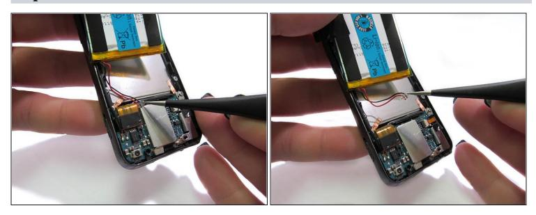
• Using pointed precision tweezers, unplug the wires connecting the battery and chip from the chip.
