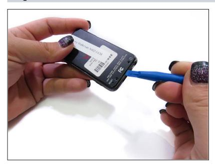
Use a small prying tool to carefully pry open the back of the device.
