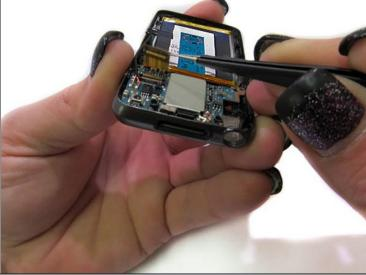
• Using tweezers, unplug the gold band connecting the device and circuit board.
