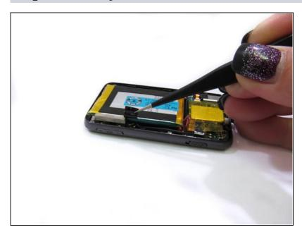
Peel back the black tape from the device to the battery from the side of the device.
