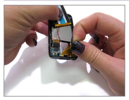
Remove the yellow film covering the circuit board with pointed precision <u>tweezers</u>.
