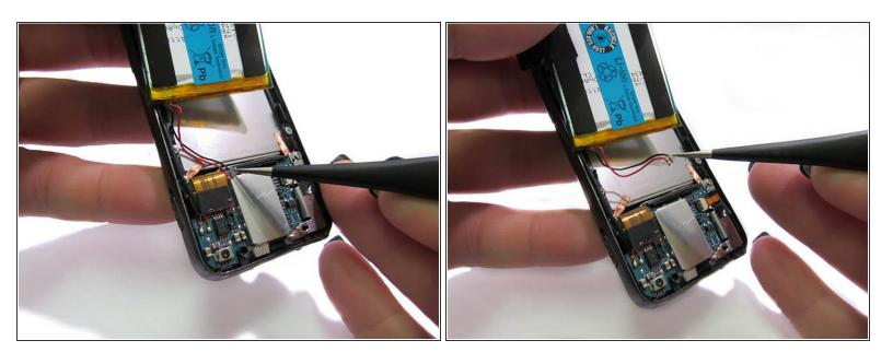
Using pointed precision tweezers, unplug the wires connecting the battery and chip from the chip.
