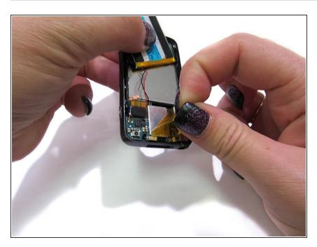
Remove the yellow film covering the circuit board with pointed precision tweezers.
