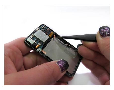
Pull up the 2 copper strips connecting the outside of the device to the inside of the device.
