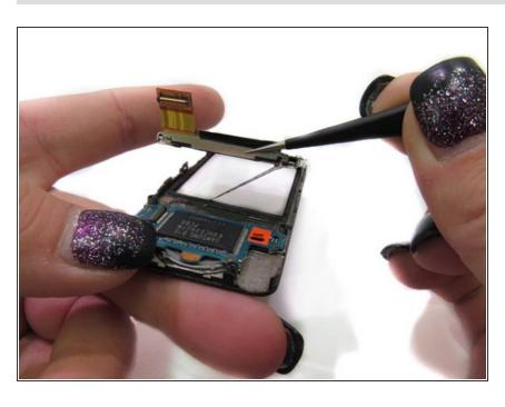
To remove screen from metal backing, use fine point tweezers to go in between the screen and metal backing and slowly pull them apart.
