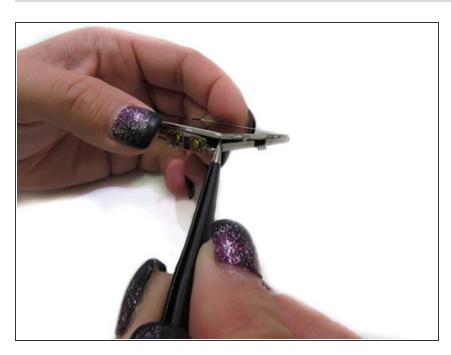
To remove the screen, use the fine point tweezers and lift up on the metal piece at the bottom of the frame.
