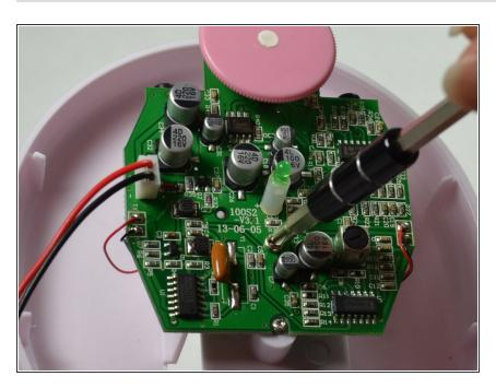
Remove the 7mm Phillips #1 screw in the middle of the motherboard.
