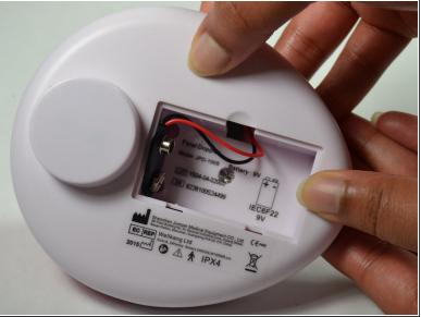
Puncture the sticker in the battery compartment with a spudger to access the screw beneath it.
