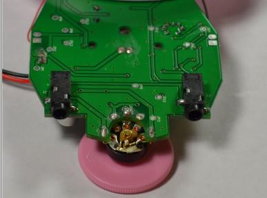
Place the motherboard in a position that allows easy access to the jacks.
