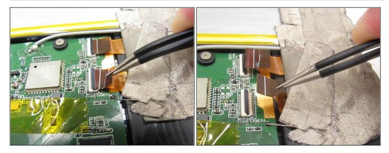
• Use <u>tweezers</u> to gently pull on both orange camera ribbons in the opposite direction in which they are connected until they disconnect from the modules on the circuit board.
