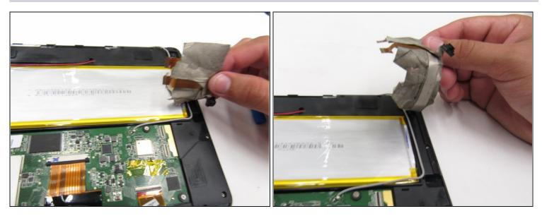
• Peel off the grey tape covering the ribbons, in order to separate the cameras and their respective ribbons from the rest of the device.
