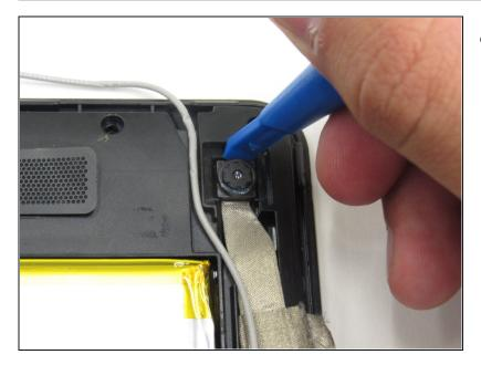
• Use a a plastic opening tool to pry out the back camera at the top of the circuit board.
