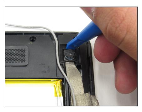
Use a a plastic opening tool to pry out the back camera at the top of the circuit board.
