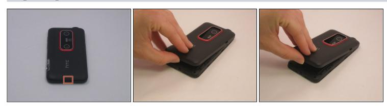
• Remove the outer casing of the phone with your hands by prying and lifting at the latch.
