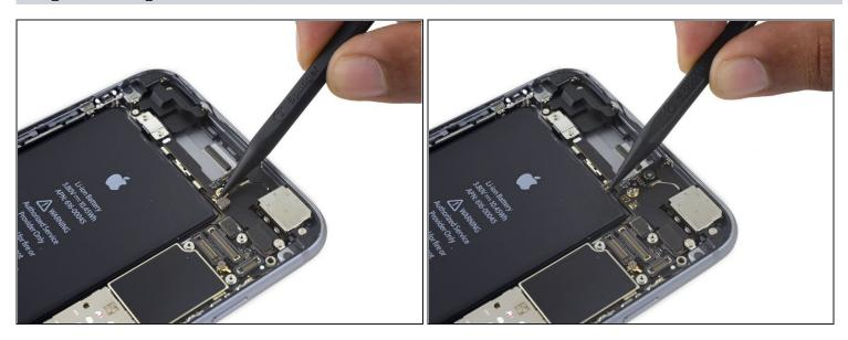
• Use the pointed end of a spudger to disconnect the top left antenna cable from the logic board.
