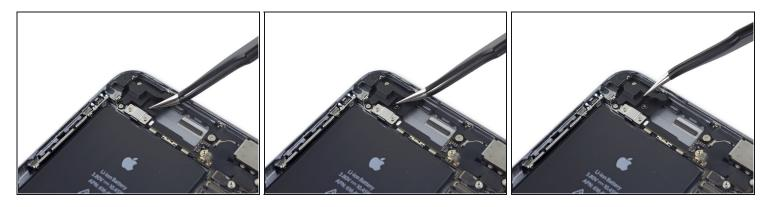
• Remove the sticker covering the third screw securing the top left antenna to the rear case.
