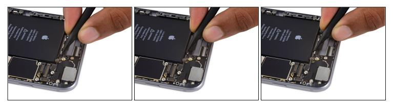
• Use the pointed end of a spudger to gently nudge the top left antenna cable out from under the rightmost clip on the logic board.
