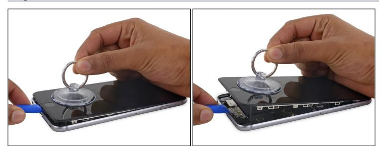
• Use a plastic opening tool to hold down the rear case while pulling up the suction cup to open the phone.
