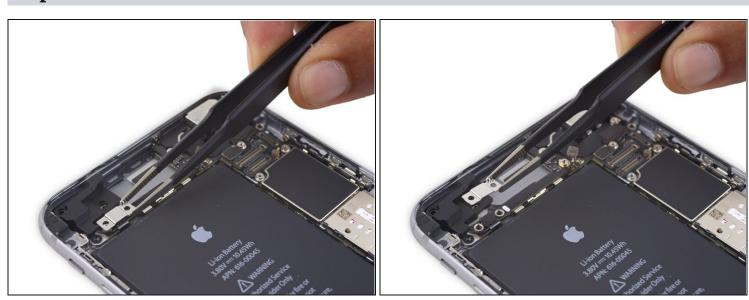
• Remove the audio control cable bracket.
