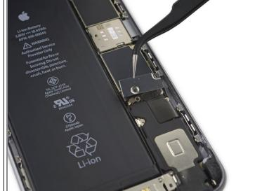
• Remove the battery connector bracket.
