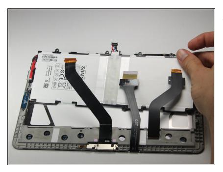
Lift the battery out of its housing to remove it.
