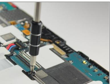
Use the Phillips #00 screwdriver to unscrew the 10 3mm screws holding the battery in place.
