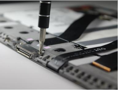
• Use the Phillips #00 screwdriver to remove both of the 3-mm screws.
