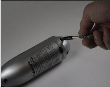
Remove three 13.3 mm Phillips PH#2 screws.
