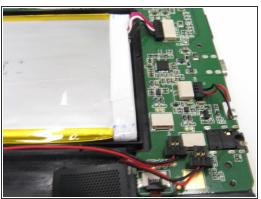
Wedge a plastic opening tool between the black and white modules on the circuit board to disconnect the wires of the speakers.
