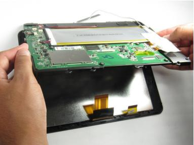
• Lift the circuit board from the screen underneath and set it aside.
