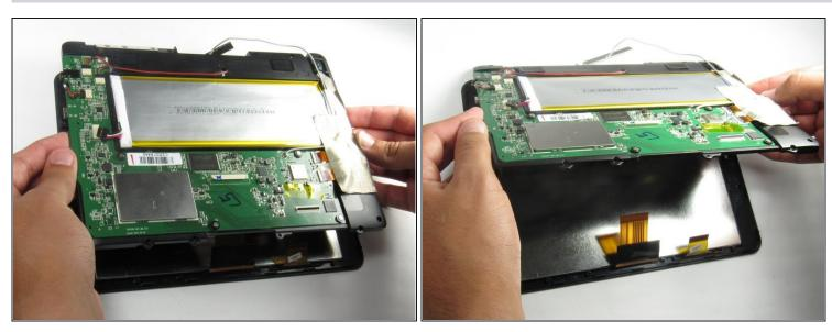
• Lift the circuit board from the screen underneath and set it aside.
