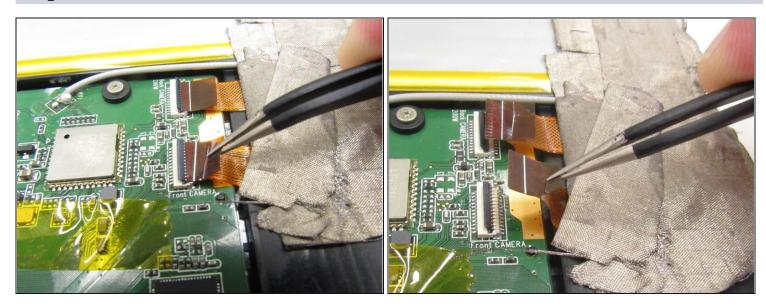
• Use <u>tweezers</u> to gently pull on both orange camera ribbons in the opposite direction in which they are connected until they disconnect from the modules on the circuit board.
