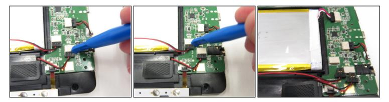
Wedge a plastic opening tool between the black and white modules on the circuit board to disconnect the wires of the speakers.
