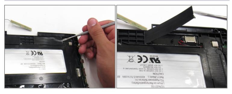
• On the back side of the circuit board, use a plastic opening tool to pry open the plastic speaker housing.
