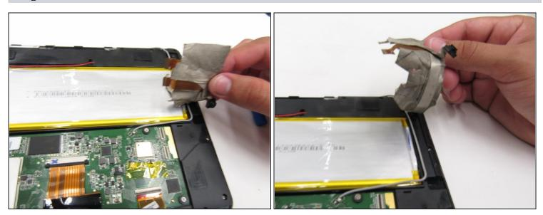
Peel the grey tape off of the device in order to separate the cameras and their respective ribbons from the rest of the device.
