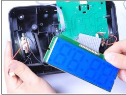
Remove the screen by pushing it toward the middle of the clock and pulling it up out of the clock.
