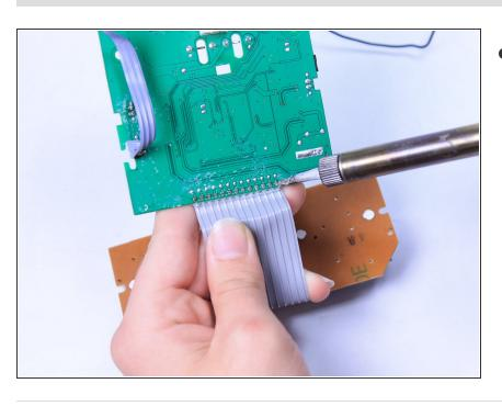
Use this <u>soldering guide</u> to remove and replace the cable and screen.
