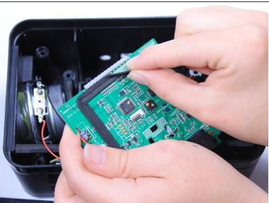
Lift the adhesive strip that covers the connections between the grey ribbon cable and the circuit board by peeling it off of the circuit board.
