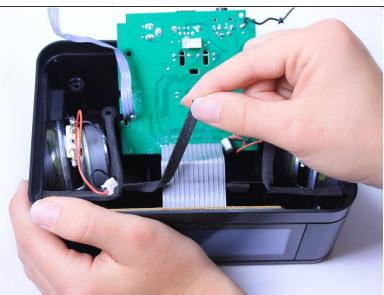
• Lift the adhesive strip that holds down the grey ribbon cable which attaches to the circuit board and the LCD screen.
