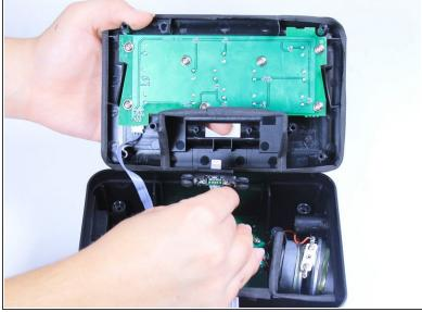
Remove the plastic casing, which encases the Apple lightning connector, from the top cover of the clock.
