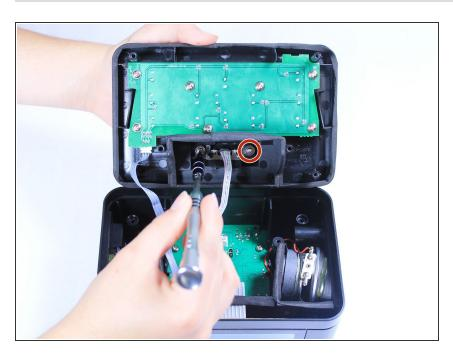
Using a Phillips #1 screwdriver, unscrew the two 7mm Phillips screws that attach the iPhone dock to the top cover of the clock.
