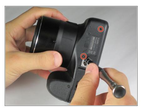
Remove 2-4 mm screws that secure the bottom of the camera using a Phillips #000 screwdriver.
