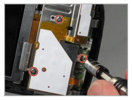
Remove 3-4.4 mm screws that secure the small metal plate using a Phillips #000 screwdriver.
