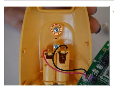
Use the Philips #00 Screwdriver to remove the 9.2 mm screw located in the middle of the back cover, above the battery compartment.
