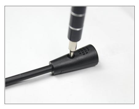
Remove the PH0 7.1 mm screw from the back casing.
