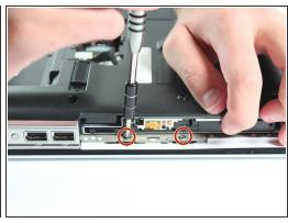
Remove the two 2.5mm screws with a Phillips #0 screwdriver.
