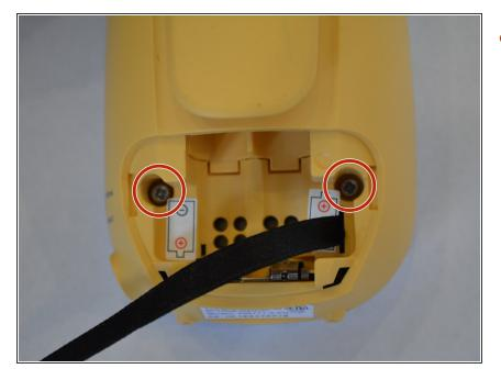
Using a Phillips #00 screwdriver, remove the two 11.2 mm Philips #00 screws located on either side of the battery slots.
