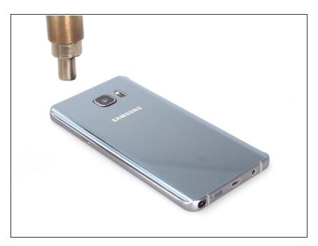
Heat the back cover to melt the strong adhesive sticker underneath.
