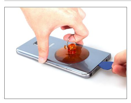
Try to pull and open a gap between back cover and frame after heat.
