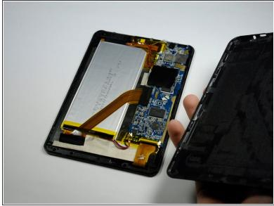
Remove the back panel from the rest of the tablet and set it aside.
