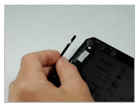
The plastic volume button cover may fall out when you remove the back panel. Set it aside.
