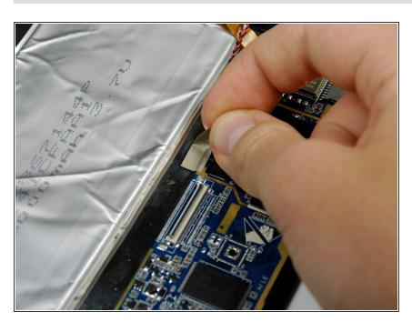
Remove the silver piece of tape from the left edge of the motherboard.
