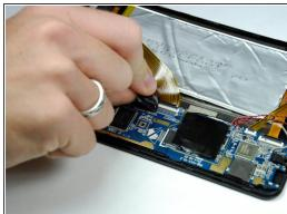
Remove the 4 pieces of tape covering the zero insertion force (ZIF) connectors on the motherboard.
