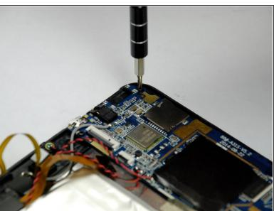
• Use a J00 Phillips head screwdriver to remove the two 4.3 mm screws securing the motherboard to the device and set them aside.
