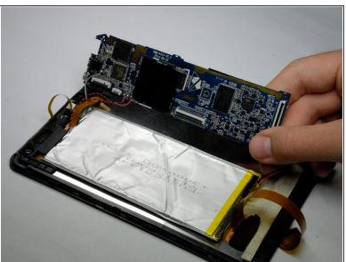
Use a spudger to lift the motherboard from the device.
