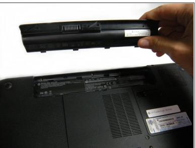
Lift the battery from its compartment away from the laptop.
