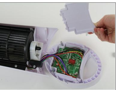
Gently lift and remove the panel covering the electronics assembly.
