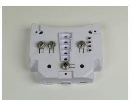
Lift out the internal part of the front panel to access the buttons.
