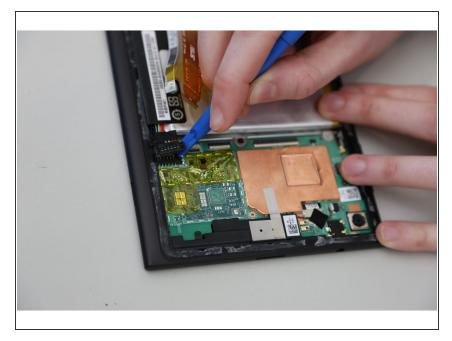
Find the place where the battery connector is. Disconnect the battery connectors by carefully pulling up on them using a spudger or plastic opening tool.
