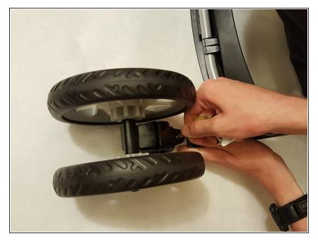
• Use a key or other thin object to push down the button holding the wheel in place.
