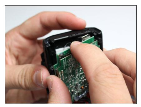
Remove the motherboard (green) from the front case housing.
