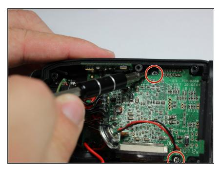
Use J0 Phillips head to remove two 6mm long Phillips head screws from the motherboard.
