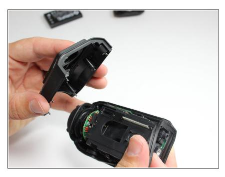
Remove the back case from camera body.
