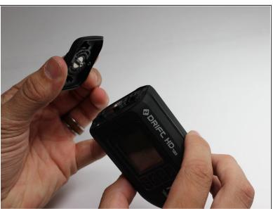
Unscrew the back plate counterclockwise until it comes off.
