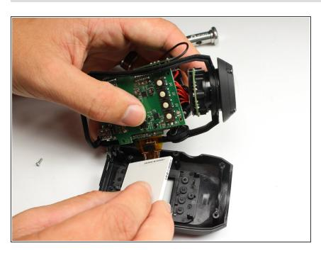
Remove the LCD screen from the front cover.
