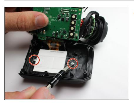
Use the J0 Phillips head screws to remove two 5mm long Phillips head screws from the plastic bracket holding LCD in place.
