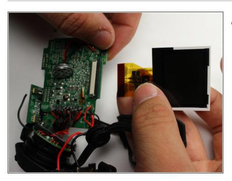
Remove the LCD from motherboard.
