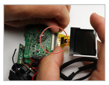
Slide the black bar toward the LCD screen in order to remove the screen from slot.
