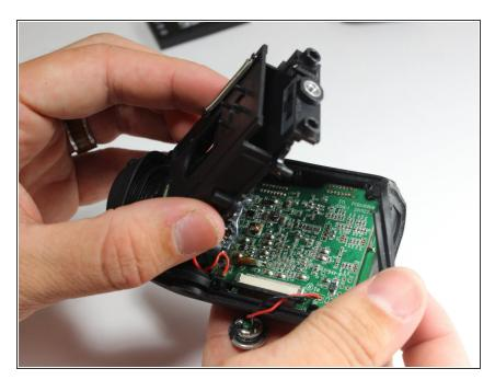
Carefully remove the battery housing from the camera body.
