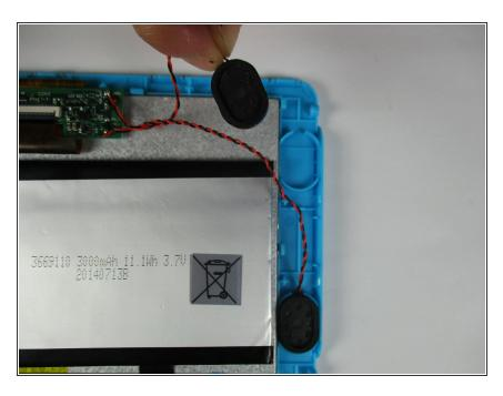
Carefully remove the speakers out of the plastic molds by lifting up the black and red wires. To reassemble your device, follow these instructions in reverse order.
