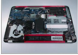
Pry open back plate area with plastic opening tool. The back plate should pry open with relative ease. If you feel some resistance at any point please refer to steps 2-5 because a screw has probably been missed.
