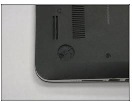
Remove the highlighted rubber stoppers with a metal spudger as pictured. They should expose a screw that you will need to remove in a later step.
