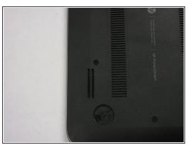
Remove plastic cover highlighted. It should expose a screw that you will need in a later step.
