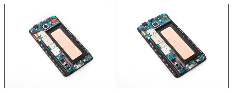
Release LCD connector, digitizer connector, earpiece assembly connector, home button connector on the motherboard.
