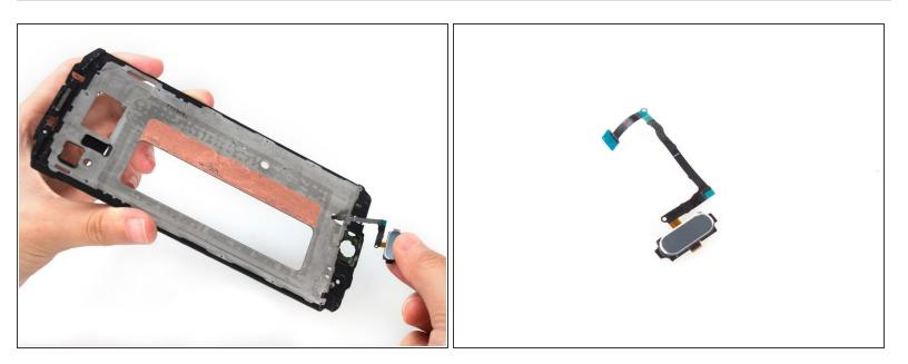
• Remove home button flex. Though it's a small component, it's really complicated and difficult to replace, even at the risk to break the screen.
