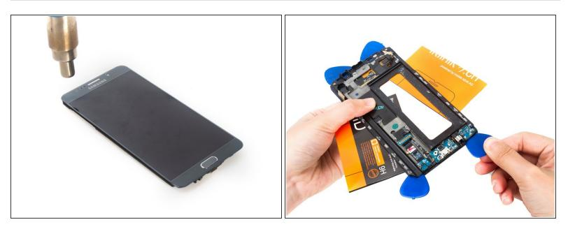
Now try to separate LCD screen from frame. The difficulty and risk to remove screen alone are getting nearly 5 stars (5 scores all together)respectively. The screen is weak and the adhesive are strong as well too much.
