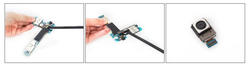
• Remove the rear camera. There is a black plastic bracket around camera. So we have to remove them together. And there is a little adhesive underlying.
