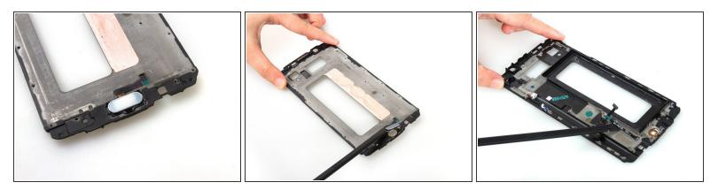
• Could you see the mark on the right of the home button? Push the button as its direction and can loosen it from securing slot easily. And then cut the adhesive sticker under the flex.
