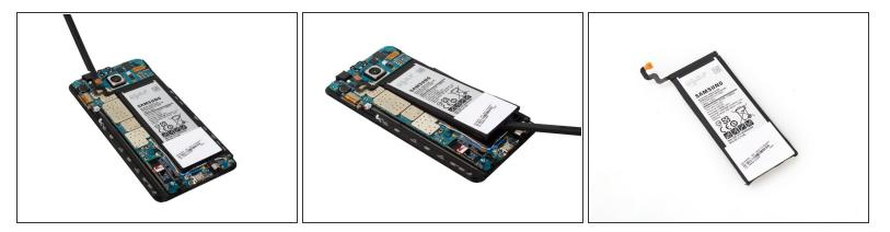
Release battery connector from motherboard and pry the battery up. Yes, there is also some adhesive underneath.
