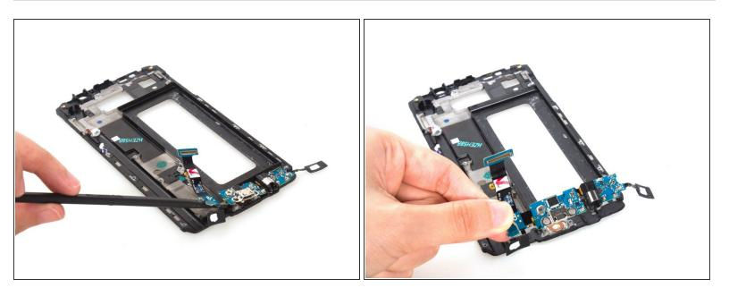
• Remove the USB board finally.
