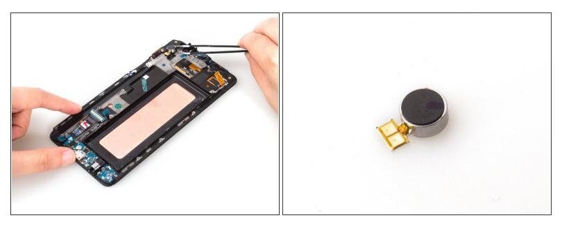
• Remove motor vibrator easily.
