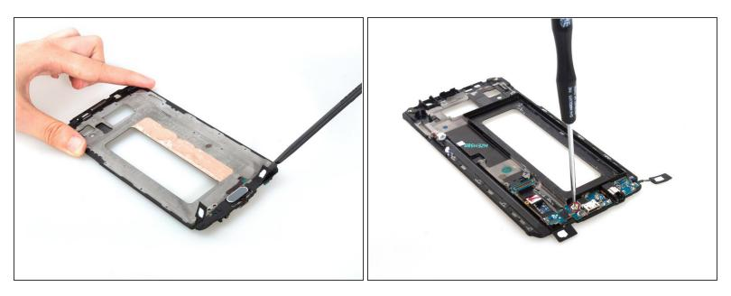
Loosen two soft sensor keys from frame carefully. And remove the last securing screw on USB board.
