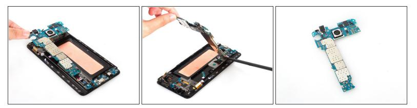
• Release USB board connector on the back and remove the whole motherboard.
