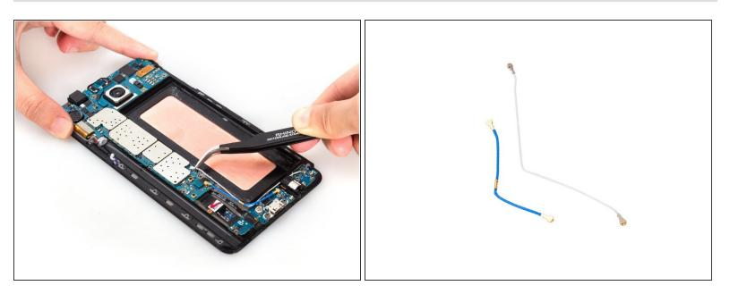
Remove two pieces of signal flex cables. And different versions Samsung Galaxy Note 5 may have only one piece signal cable.
