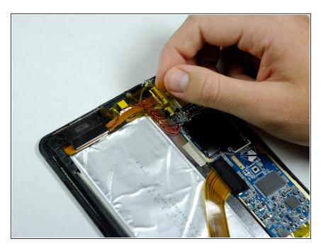
Remove the yellow tape covering the set of wires located near the upper right corner of the battery.
