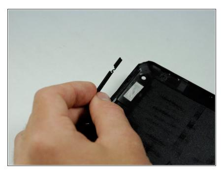
The plastic volume button cover may fall out when you remove the back panel. Set it aside.
