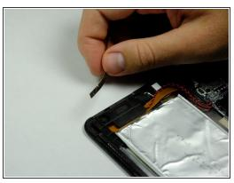
Use your fingers to carefully peel the volume sensors away from the top of the plastic L-shaped speaker housing.
