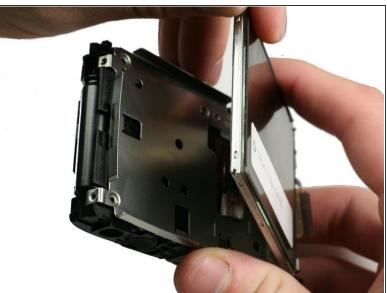
Remove the LCD screen from the metal mount.
