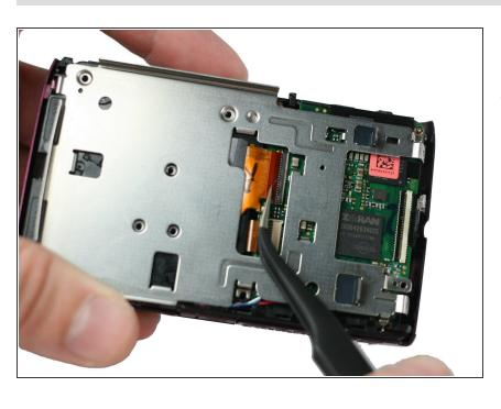
Using precision tweezers, grab the base of the first ribbon cable and pull out parallel to the metal mount.
