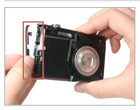
Remove the remaining side shell casing.
