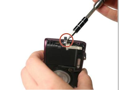
Using the Philips #000 head screwdriver, remove 2 additional 3.30 mm screws holding the lanyard mount in place.
