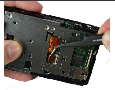
Using precision tweezers, grab the base of the second ribbon cable and pull out parallel to the metal mount.
