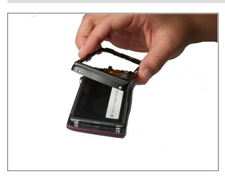
Remove the black casing on the back of the camera that runs around the LCD screen.
