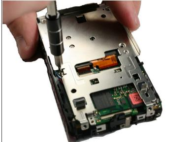
Using a Philips #000 head screwdriver, remove 7 Philips head screws of length 3.4mm from the metal LCD camera mount.
