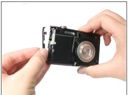
Remove the lanyard mount and accompanying side shell casing off of the camera.
