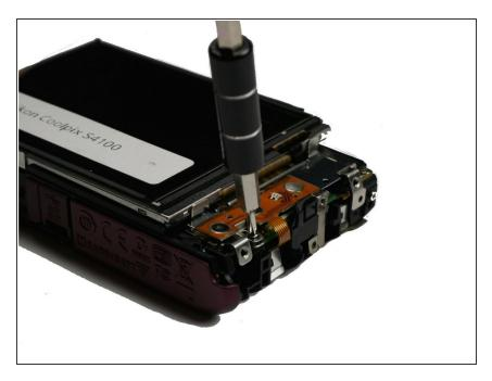
Using the Philips #000 head screwdriver, remove the 3.40 mm screw located near the functional buttons.
