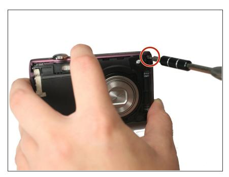
Using the Philips #000 head screwdriver, remove the 3.40 mm screw located on the front of the camera in the upper corner by the LED light.
