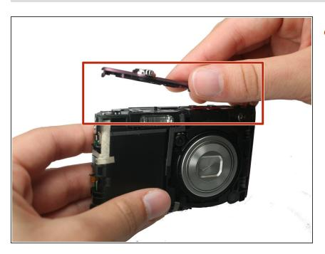
Remove the top shell casing.
