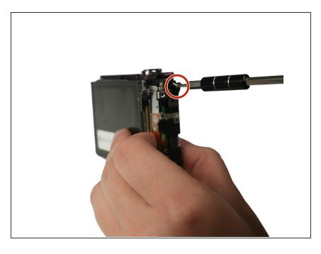
Using the Philips #000 head screwdriver, remove the 3.30 mm screw securing the top shell casing.
