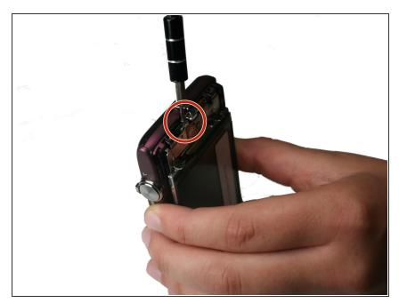
Using the Philips #000 head screwdriver, remove the 1.90 mm internal screw located just above the lanyard mount.
