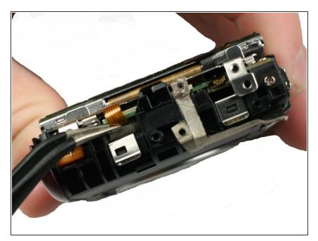
Using precision tweezers, remove the ribbon cable that runs from the functional buttons plate to the under side of the motherboard.
