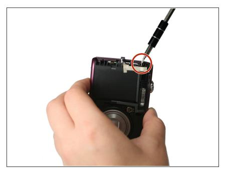
Using the Philips #000 head screwdriver, remove the 3.30 mm screw located on the side of the camera near the lanyard mount.
