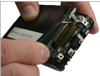
Using precision tweezers, gently remove the ribbon cable running from LCD to the bottom side of the motherboard.
