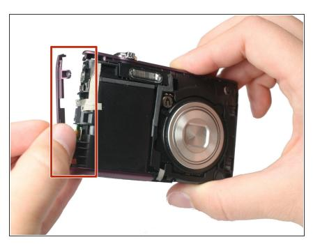
Remove the remaining side shell casing.
