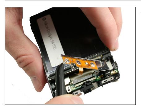
Using precision tweezers, lift up the bottom of the functional buttons plate and remove the metal plate.
