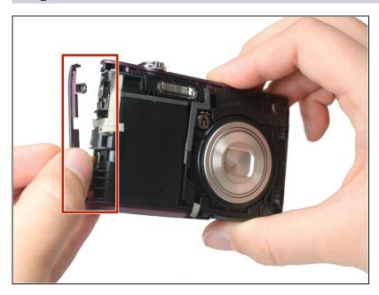
• Remove the remaining side shell casing.
