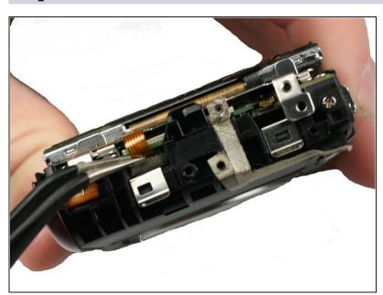
Using precision tweezers, remove the ribbon cable that runs from the functional buttons plate to the under side of the motherboard.
