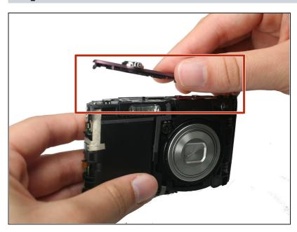
• Remove the top shell casing.
