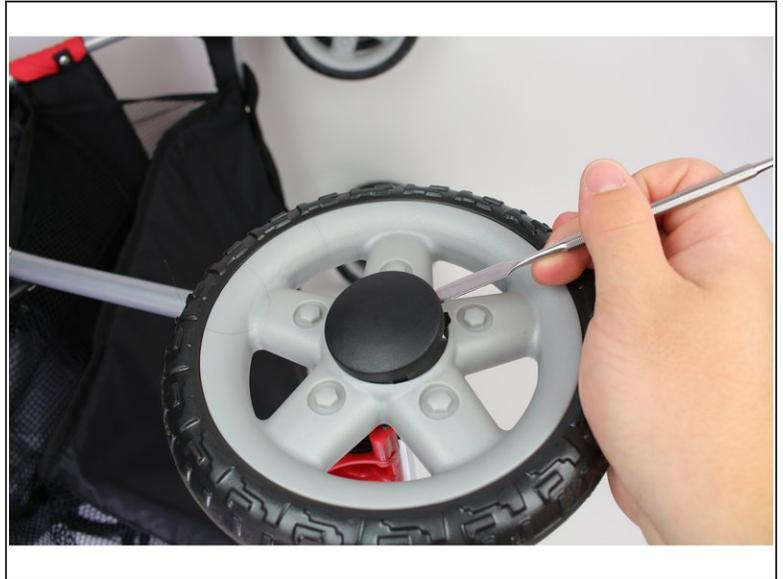
**!** Applying too much force to the spudger can cause the spudger to bend or the hubcap to break. To avoid this, try prying the hubcap from a different angle or positioning your spudger at a different points around the hubcap.
