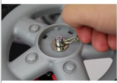
Pull on the looped end of the cotter pin to remove it.
