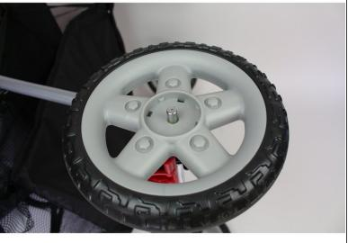
Remove the metal washer by sliding it off the axle.
