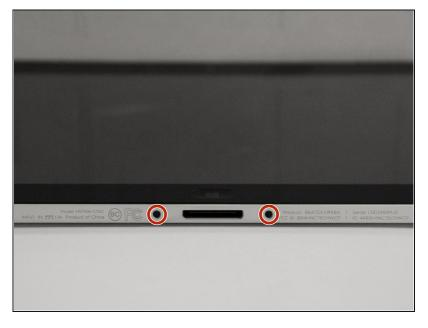
Unscrew the two 2.8mm Phillips #000 screws near the power connector.
