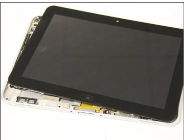
Use a suction cup to pull the display assembly up.
