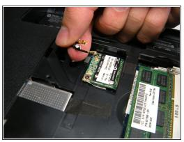
• Unlatch the two antenna cable connectors from the wireless card.
