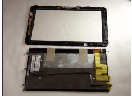
• Use a plastic opening tool to separate the LCD from the digitizer.
