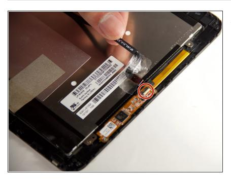
Use the tip of a spudger to disconnect the ribbon cable ZIF connector.
