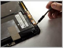
• Remove the four 1.6mm Phillips #000 screws securing the LCD to the digitizer.
