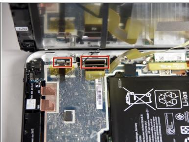
Use the tip of a spudger to disconnect the two display <u>ZIF connectors</u>.
