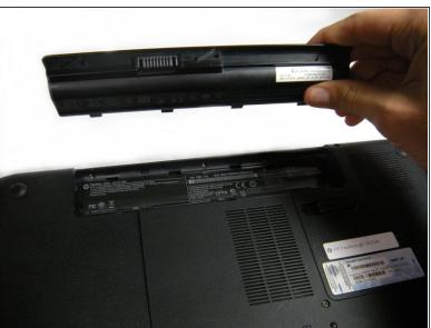
Lift the battery from its compartment away from the laptop.
