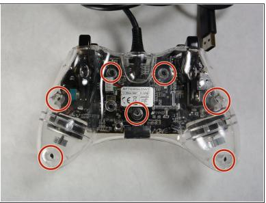
Loosen the seven 11 mm Phillips #0 screws located on the back of the controller.
