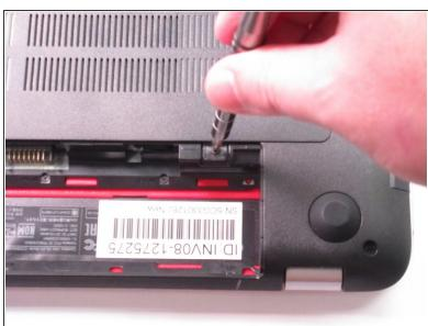
Remove the single screw holding the accessory plate. This is a PH0 2.0x2.5 screw.
