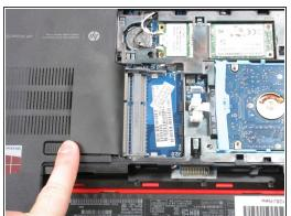
You can now remove the RAM modules you need to replace. You can replace the top one, the bottom one, or both if needed.
