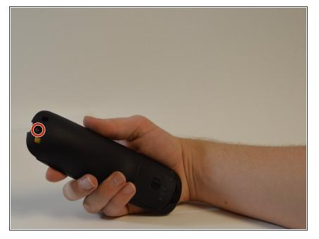
Remove the single 6 mm Phillips #0 screw located beneath the sticker near the USB charging port.
