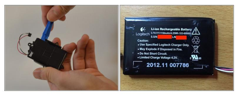
• Use the plastic opening tool to separate the battery from the case.
