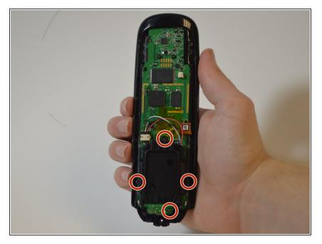
Remove the four 6mm Phillips #0 screws from the battery case.
