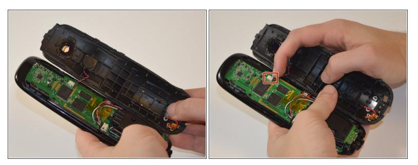
Disconnect the wires running from the back cover to the motherboard.
