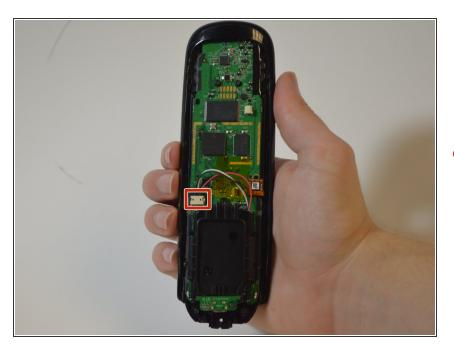
• The battery is still connected to the device via wiring. To free the battery completely, remove the dark plastic piece from the slot with the plastic opening tool. Slowly rotate the dark plastic piece and the battery clockwise until then can be removed from underneath the small circuit board with the USB port.
