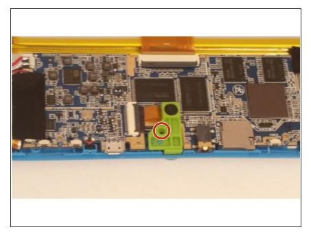
Remove the single screw attaching the camera to the device.
