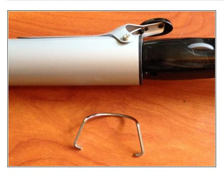
Use your fingers to pull the ends of the stand away from the barrel. The metal stand should be easy to pry from the sides of the barrel.
