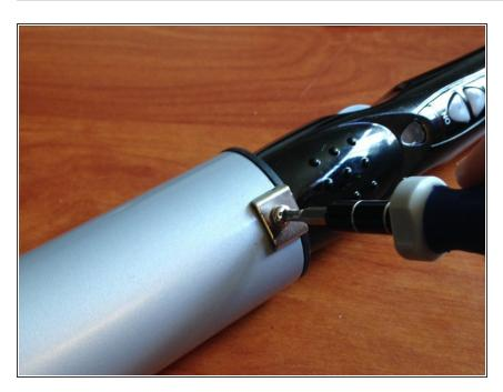
Using a 3mm Flathead Screwdriver, remove the screw holding the spring plate in place.
