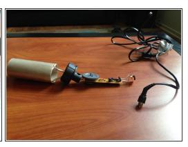
Using your hands, slowly pull the cord away from the socket. The cord should easily slide out of the socket.
