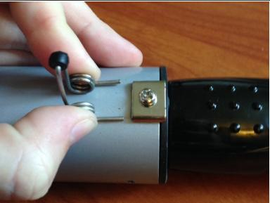
Using two fingers, squeeze either side of the spring and slide the ends away from the barrel.
