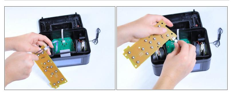
Detach the circuit board from the rest of the clock by gripping the sides of the white ribbon cable connector on the left-hand side of the board and pulling it straight off. You may need to use tweezers to grip the connector.
