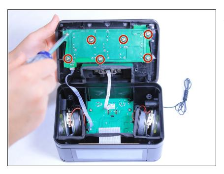
Using the Phillips #2 screwdriver, unscrew the seven 6mm Phillips screws on the circuit board that is attached to the top of the case.
