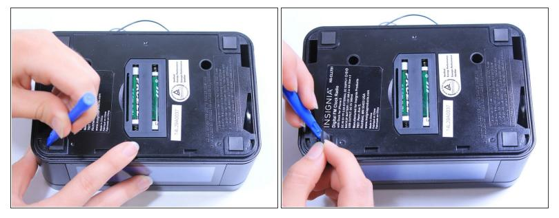
Lift the four adhesive covers on each of the corners on the bottom of the clock using a plastic opening tool or your fingernail.
