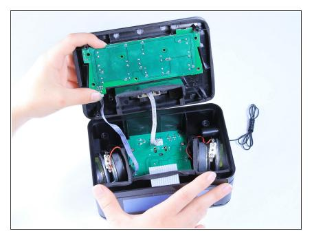
• Lift the circuit board from the device.
