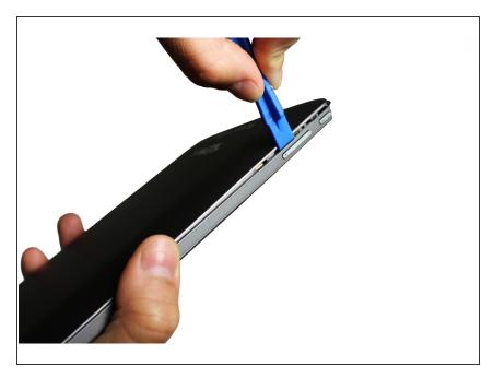
Use the plastic opening tool to work your way around the tablet, releasing the back case from the tabs.
