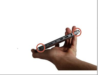
• Remove the (4) 3.5mm screws using a phillips #000 screwdriver.
