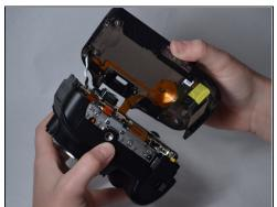
• Once all screws have been removed, carefully pull the casing apart. Take care not to pull any wires apart.
