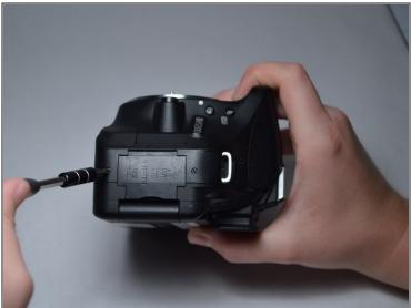
• Remove the 7-mm screws from either side of the camera.
